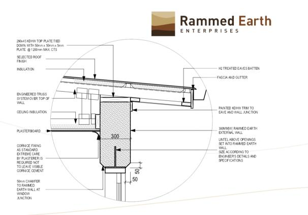
*Note.* The above contents pertain to walls built by Rammed Earth Enterprises Pty Ltd. These diagrams have been cropped and are not to scale.
